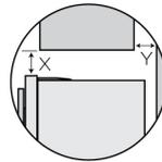
If you have a cupboard above the refrigerator with a rear gap of less than 100mm (Y), recommended minimum clearance at the top of the refrigerator increases from 30mm to 70mm (X).
