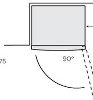
When positioned in a corner area, clearance of at least 350mm on the hinge side will allow the doors to open enough to enable the removal of the bins and shelves.
